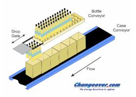
While the bottles are staging, an empty case is positioned under the staging area or drop grid. This case is often raised so as to minimize the vertical drop from staging to the case bottom. Some designs lower the case as the bottles drop reducing the shock. Once case and bottles are in position, the gate is opened and all products drop simultaneously into the case. Fingers between each bottle help guide them into position as they fall.
