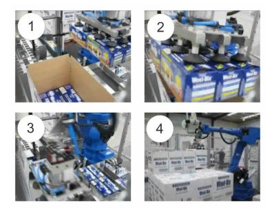
In a vertical placing system the product is must first be collated and isolated in a staging area. A 4 X 3 pattern for vertical pickoff can be collated by dividing the flow of products into 3 lanes, then using hold-backs to release backpressure on the last 4 products in each lane. The robot arm, with 12 grippers or suctions cups, picks up the entire pattern and places it in the case
