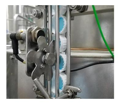
In all cases it is generally a good idea to have a sensor on the cap chute to detect misoriented caps before they cause a jam at the escapement. Some machines use photoeyes or other electronic sensors. This petal design is mechanical and simple. The sensor shown is for alarm but is not strictly necessary. In the event of an upside down cap the petal will jam. A cap presence sensor near the escapement will sense an absence of caps and stop the capper.
