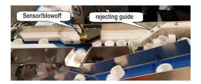
Step feeder Courtesy Performance Feeders Inc
