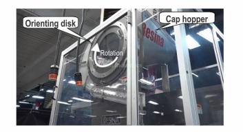
Vertical disk cap feeder (Courtesy Frain Industries)
