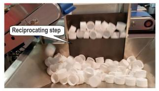
Step feeder Courtesy Performance Feeders Inc
